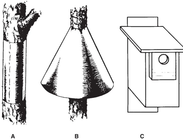
**Figure 3. Predator guards: A and B, sheet metal; C, raccoon guard (extra piece of wood around entrance hole makes it difficult for paws or beaks to reach nest).**
