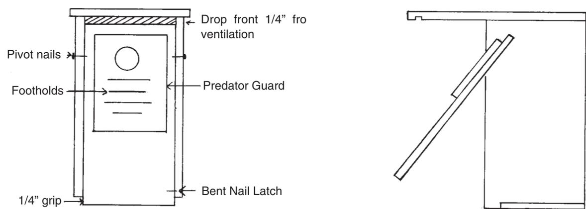
**Figure 1. Plans for a basic bird box. It takes only 30 inches of 3/4" x 10" exterior plywood to make one box. Attach to tree or pole with twisted coat hanger wire. Use information in Table 1 to modify floor plan to accommodate larger species.**
