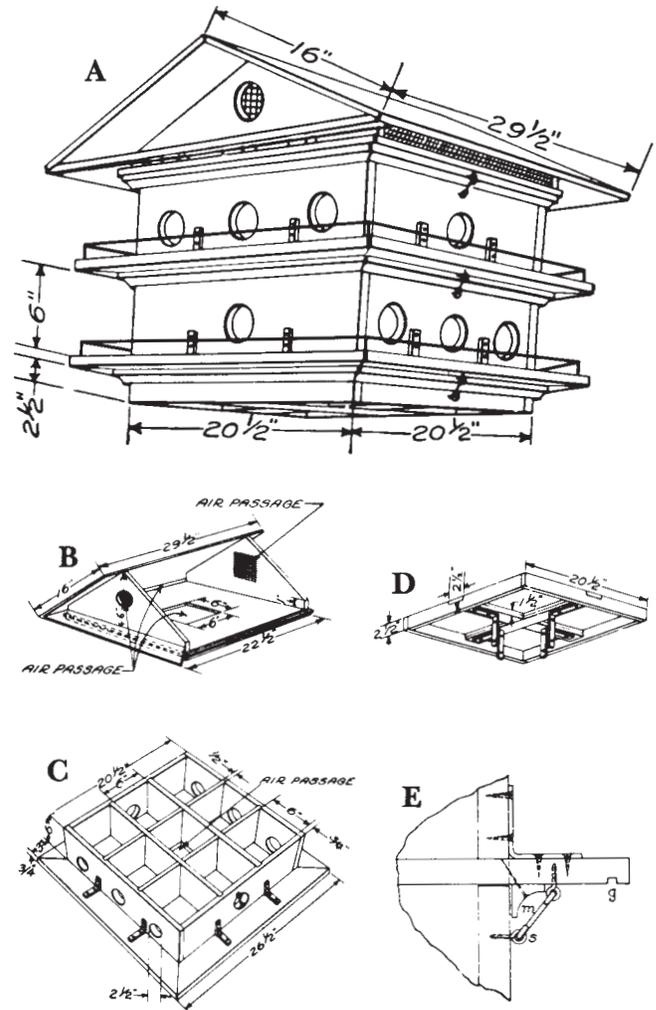
**Figure 2. A, The completed martin house; B, Details of attic designed for ventilation; C, Floor plan for each level of the house. Remove floor from center chamber. D, Foundation - note double thickness of central cross (3/4" stock); E, Detail of porch. Note rain groove (g).**
